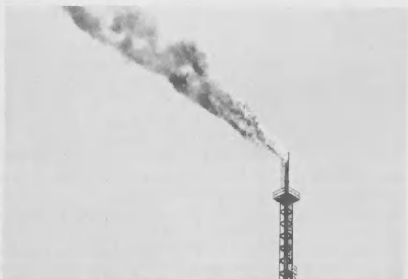
BRILLIANT FLAMES indicative of flares are a common sight throughout the refining world. Flares are part of vast safety network that is effected during unit emergencies.
